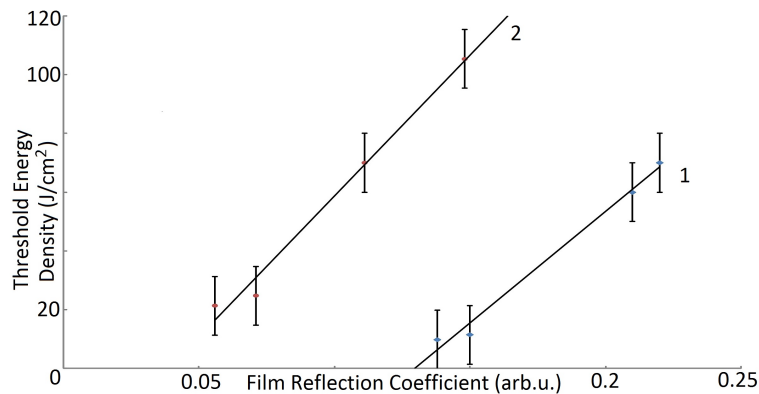
FIG. 4. The plots of the laser ablation destruction threshold energy density of F_{bn} dependence on the composites light transmission in the visible range of T . The line 1 – a one-layer film, line 2 – double-layers one. Drawing speed – 3.8 mm/s
